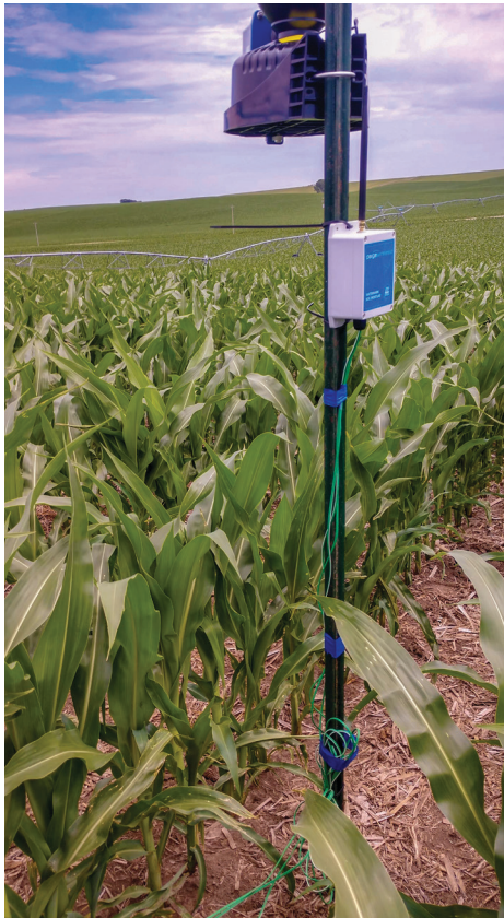
Soil moisture sensors help farmers to accurately determine when their fields need to be irrigated without fear of overwatering or leaching expensive inputs out of the crop root zone. Photo credit John Krohn.
