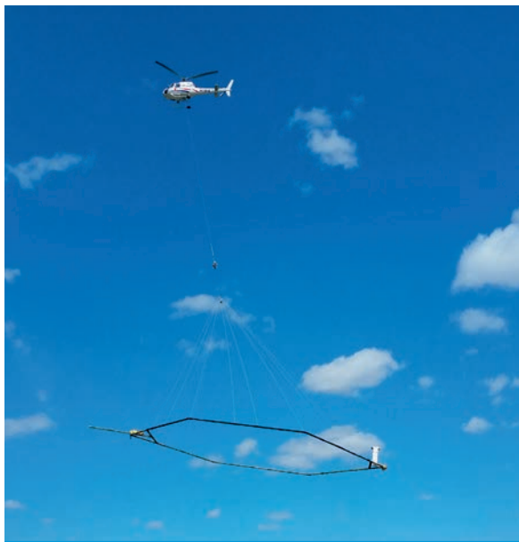
AEM flights are captured by a helicopter towing survey equipment.
