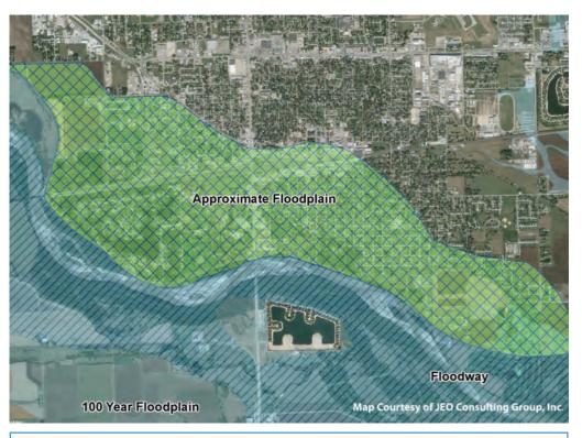
The map above shows the approximate expanded floodplain in Columbus that would exist without the recertification of the Loup River Levee.
