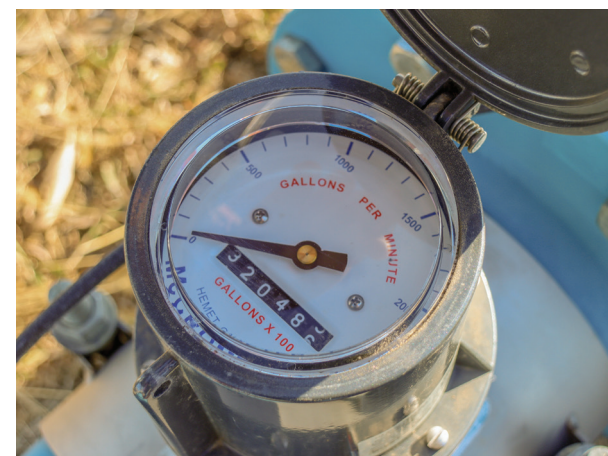
Example of a flow meter that records in gallons per minute.
