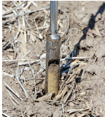
Hand operated soil sampler.
