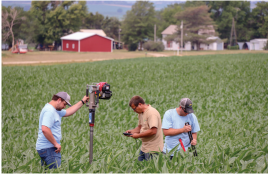
Technicians from the Lower Loup NRD collect vadose zone samples near St. Edward.
